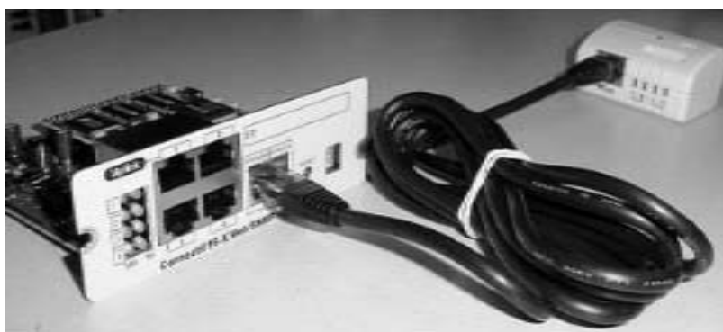
Figure 25. ConnectUPS-X Web/SNMP Module and Environmental Monitoring Probe.
